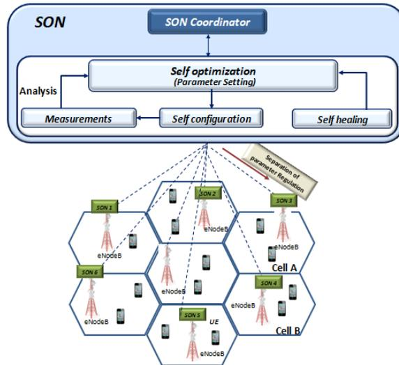
**Fig. 9.** SON coordination with Separation of Parameter Regulation
