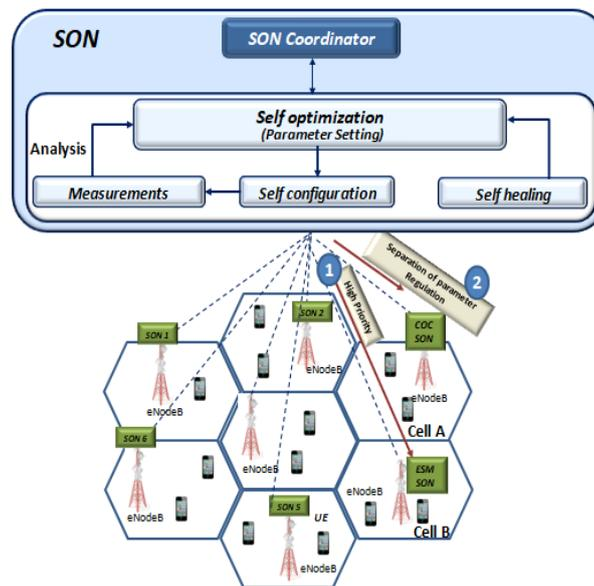
**Fig. 10.** SON coordination with Priorities for Separation of Parameter Regulation
