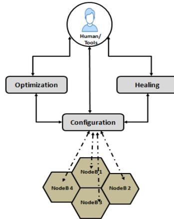
**Fig.1.** Manual efforts of optimizing network parameters in NodeBs
